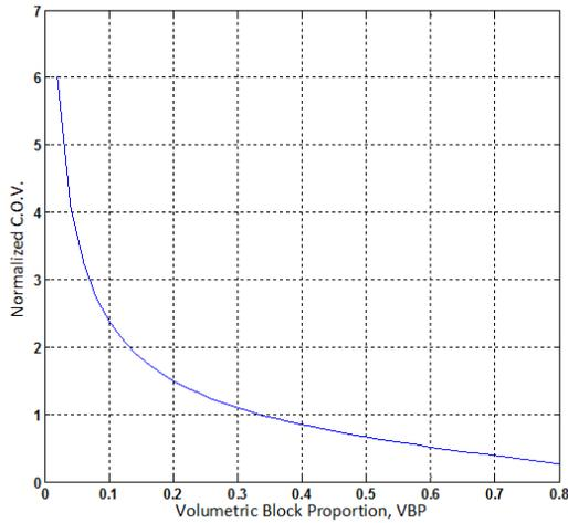
Figure 6 VBP versus normalized C.O.V. plot.
