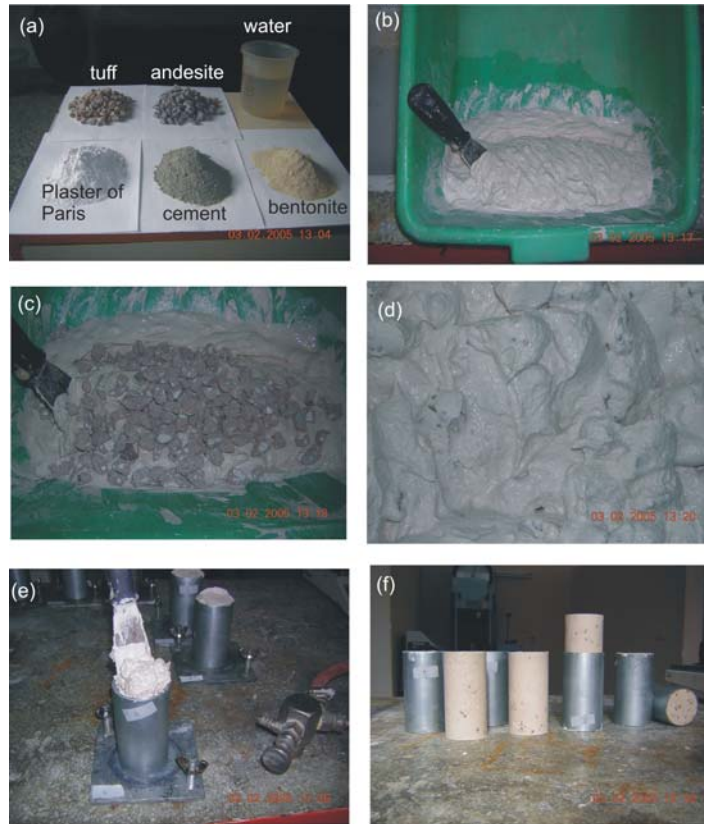
Fig. 2. Preparation stages of the artificial bimrock.
