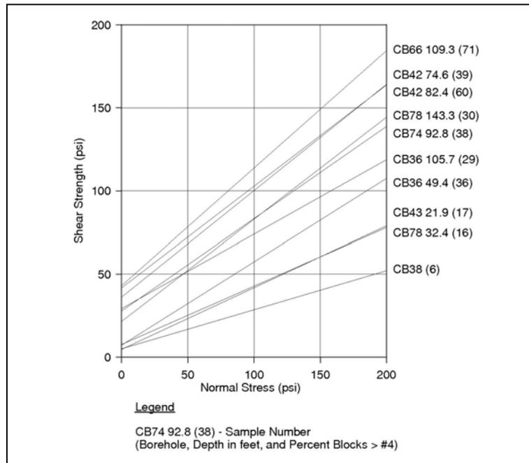
Figure 6. Results of Triaxial Tests With Block Proportions
