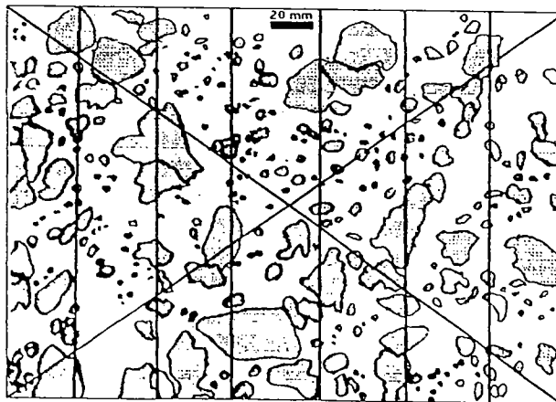
Figure 2: Graphic model of melange with scanlines. Scale bar is 20 mm long
