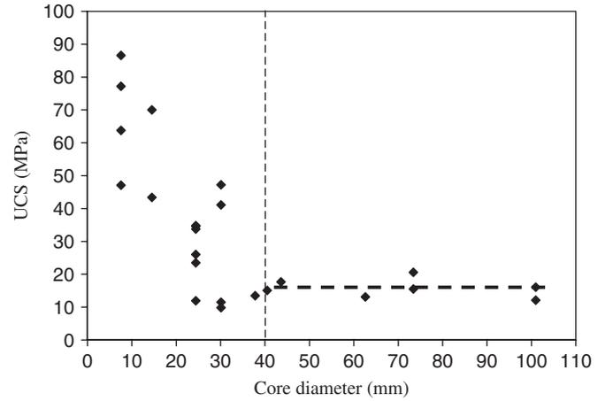
Fig. 14. UCS versus core diameter (high UCS for small diameter cores reflects bias to successfully sampling component because bimrock would full apart).
