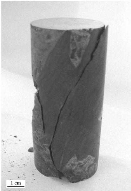
Fig. 10. Failures through blocks in the sample having large blocks and block size  $> 75\%$  of characteristic engineering dimension (VBP = 74.6%, diameter = 30.1 mm).
