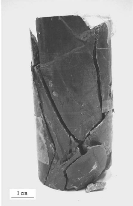
Fig. 9. Failures through blocks in the sample having a VBP of 88.2%.
