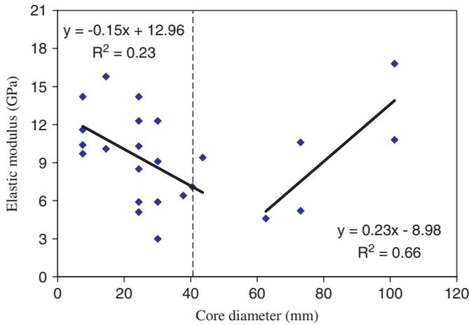
Fig. 19. Elastic modulus versus core diameter.
