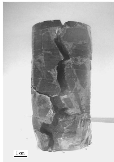
Fig. 8. Failure plane passing around block boundaries (VBP = 70.7%).
