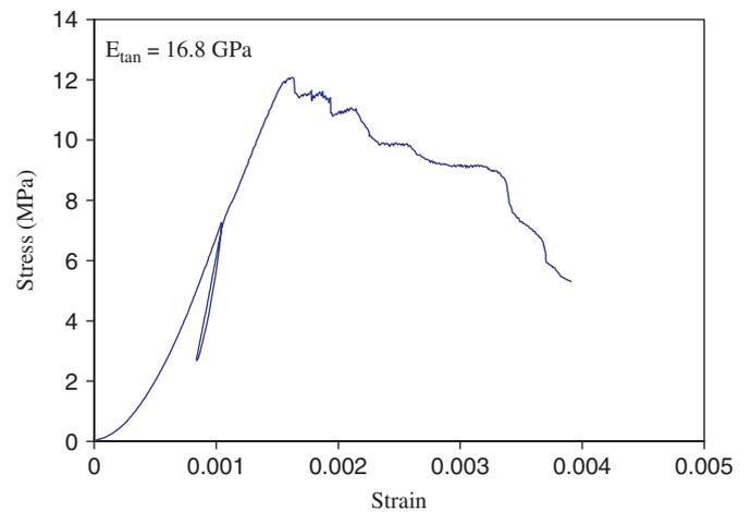
Fig. 12. Stress-strain diagram for sample no. 1 (101.3 mm-diameter).
