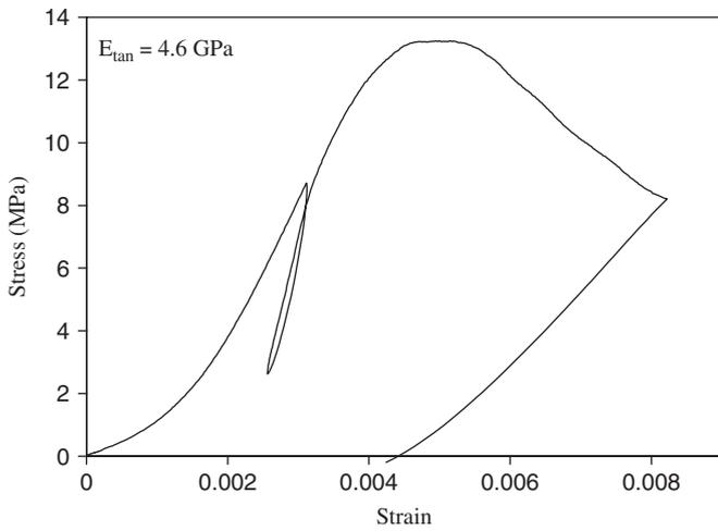
Fig. 13. Stress–strain diagram for sample no. 3 (62.6 mm-diameter).
