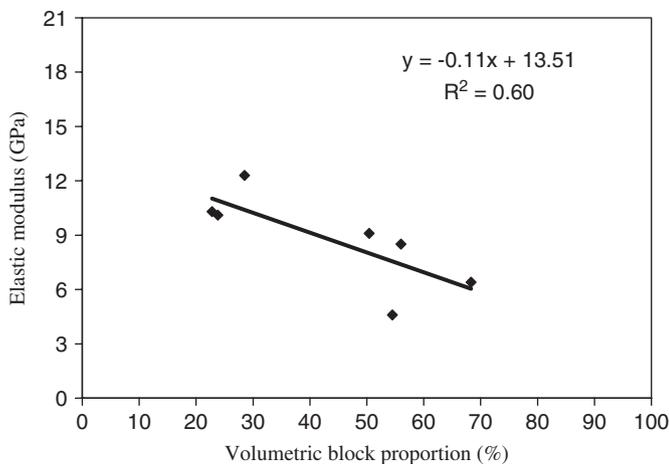
Fig. 21. Elastic modulus versus VBP for about 20% and 70% VBP.
