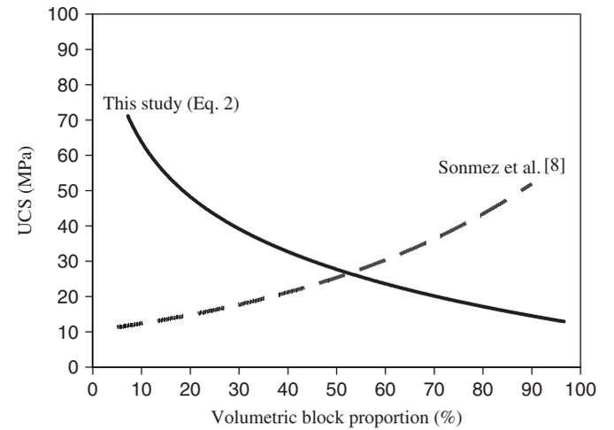
Fig. 18. Schematic comparison between Eq. (2) and the equation derived by Sonmez et al. [8].
