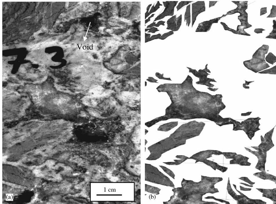
Fig. 5. Original (a) and processed (b) images of a sample having a VBP of 23.1%.
