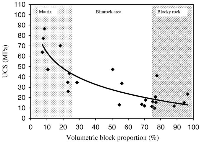
Fig. 16. VBP versus UCS (Matrix, bimrock and blocky rock areas are shown according to Medley [2]).
