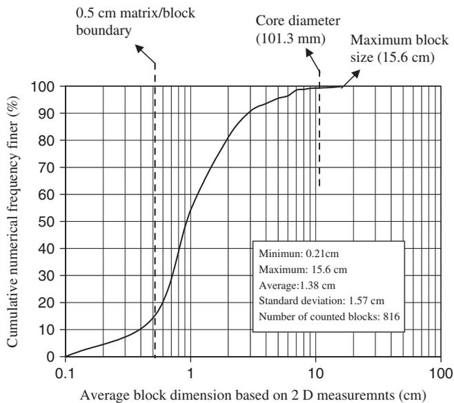
Fig. 6. Block size distribution of the breccia from scanned images of the original twelve 101.3 mm-diameter-cores.
