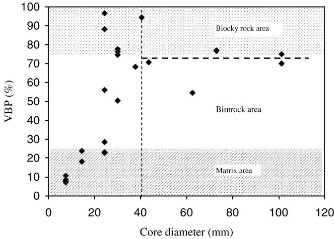
Fig. 15. Volumetric block proportion (VBP) versus core diameter (Matrix, bimrock and blocky rock areas are shown according to Medley [2]).
