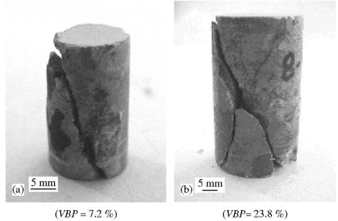
Fig. 11. Failure dominantly through matrix in the samples having low VBP.
