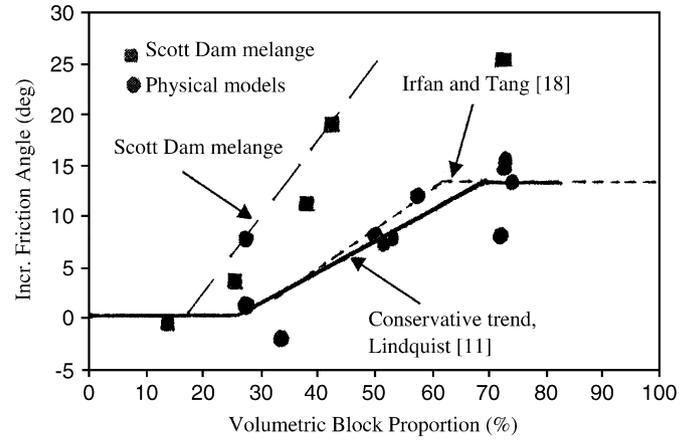
Fig. 17. Relation between friction angle and volumetric block proportion (after Medley [17]) [11,18].
