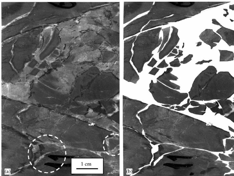
Fig. 4. Original (a) and processed (b) images of a sample having a VBP of 76.3%. The blocks in the circles are the fragmented pieces of larger blocks separated by infilled joints.
