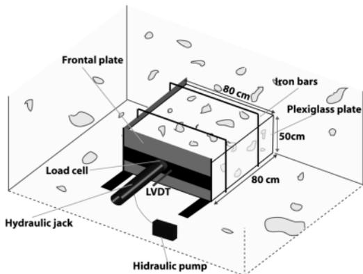
Figure 2. Schematic representation of the shear test apparatus.
