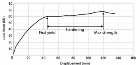
Figure 4. Double yield force-displacement curve of test P3.
