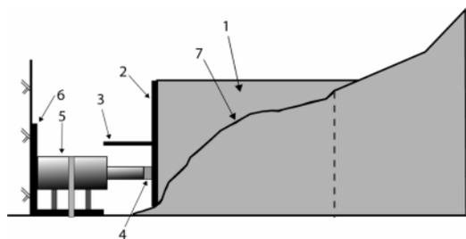
Figure 3. Testing scheme. 1) specimen, 2) frontal steel plate, 3) LVDT transducer, 4) load cell, 5) hydraulic jack, 6) support plate and holder for the hydraulic jack, 7) failure surface.
