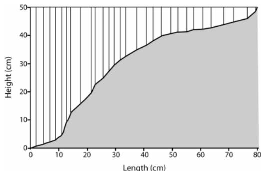
Figure 5. One of the four cross section of test P3. The upper sliding area is subdivided into several slices.
