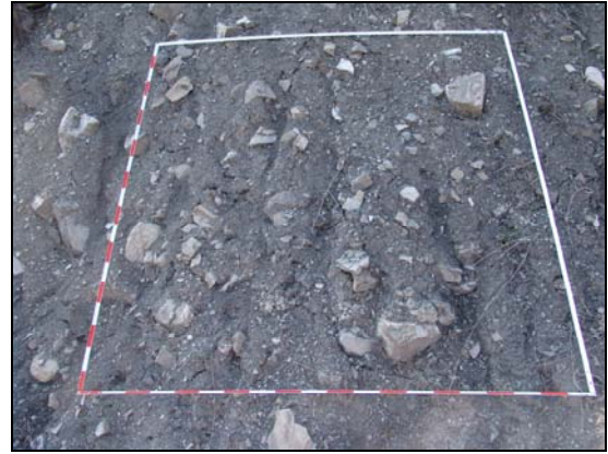
Fig. 5. Example of a photographic shot on a natural SLCC outcrop (the aluminium square reference frame is 2 m x 2 m).
